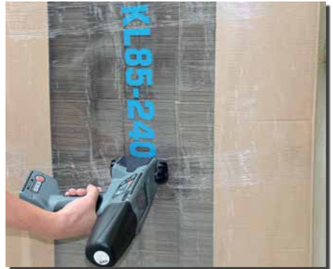
Prints on stretch wrap with pigmented ink
